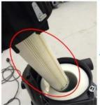
When fitting the motor pack onto the cyclone, make sure the HEPA filters stays in place. — As highlighted
